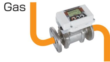
The flow meter has to be located 10D or more distant from a governor irrespective whether it is placed upstream or downstream of the governor. Failing to meet this condition may lead to inaccurate measurements. (D = pipe diameter)
